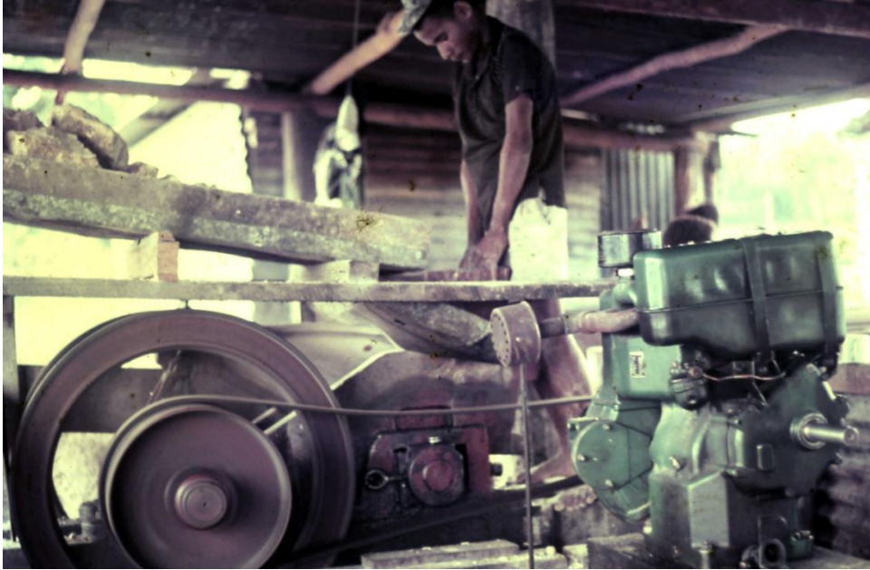
Crushing the limestone for our next stage—brick-making.
